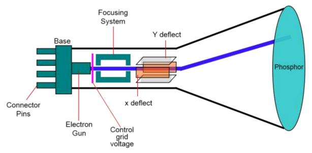
Figure: Cathode Ray Tube
